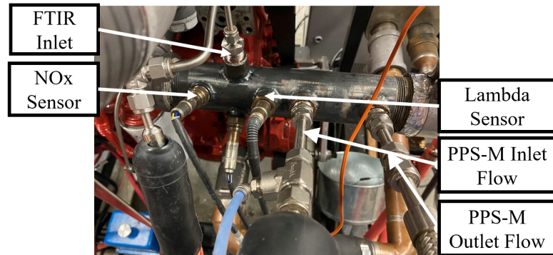
Figure 2.3: Diesel engine exhaust pipe– The FTIR, PPM, \text{NO}_x , and Lambda sensor are mounted in this pipe
